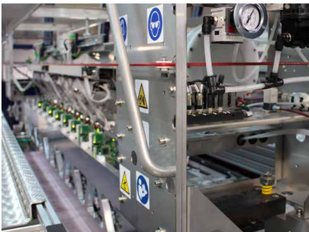
Since the printing heads on the MS LaRIO are fixed, there can be no loss of alignment as the ink is dispensed, which helps eliminate printing errors.
